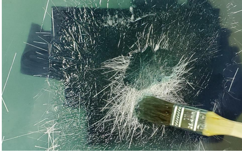
Figure 38: Soak Fiberglass with Paint Brush
