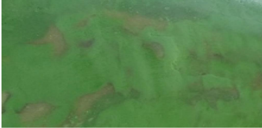
Figure 47: Fiberglass Visible Through Putty Repair, Needing Gelcoat Repair
