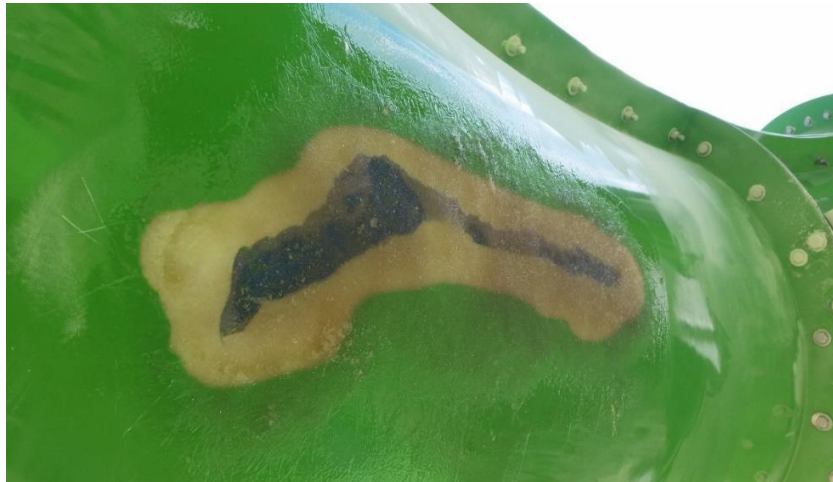
Figure 39: Cured Fiberglass Repair, Outside
