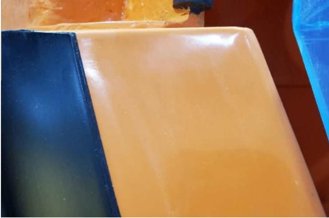
Figure 67: Buffed Small Putty Repair
