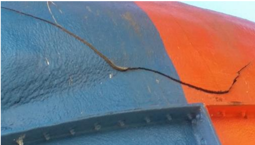
Figure 14: Crack in FRP
