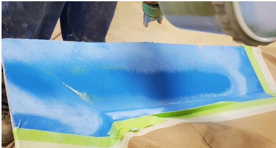
Figure 53: Spray on an Even Coat
