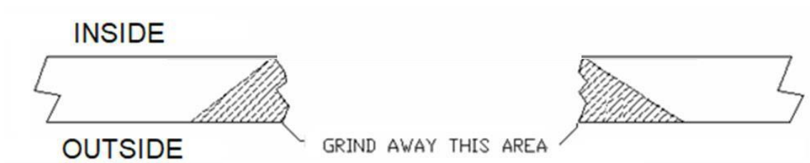
Figure 28: Grind Away Repair Area
