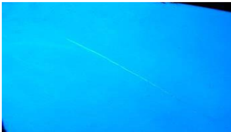
Figure 19: Gouge in AquaLucent FRP
