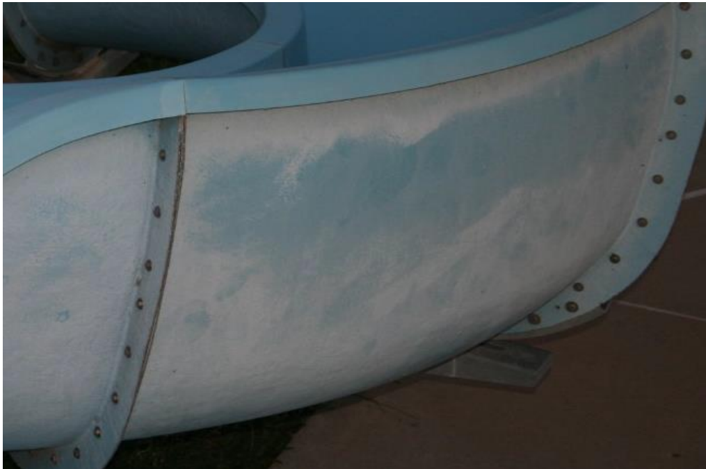
Figure 24: Faded Clear Coat DC92
