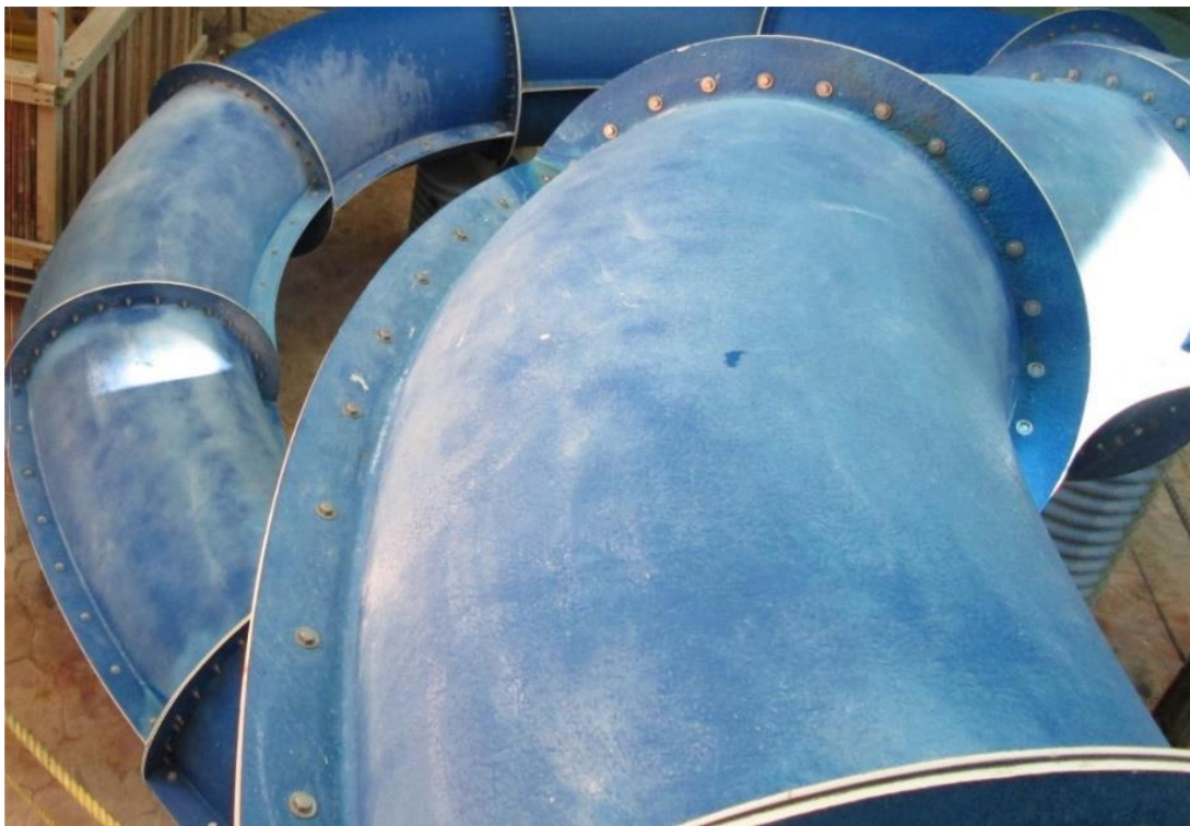
Figure 2: UV Radiation Effects on FRP
