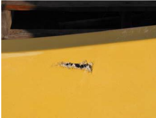
Figure 15: Puncture Holes in FRP
