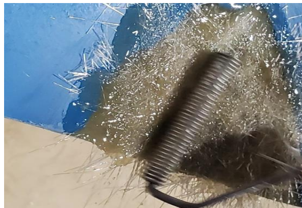
Figure 37: Smooth Out Air Bubbles with Metal Roller
