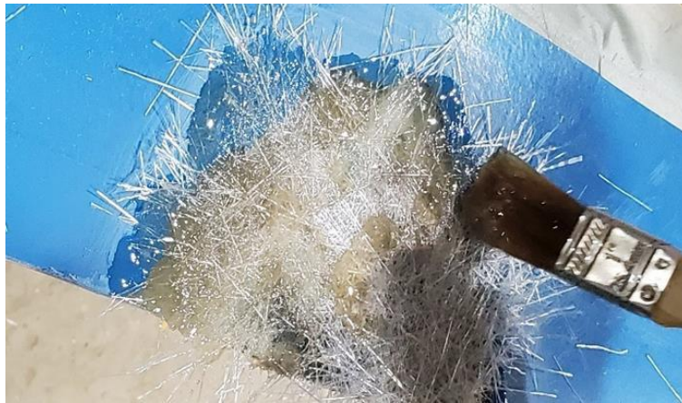
Figure 36: Use Paint Brush to Soak Fiberglass with Resin
