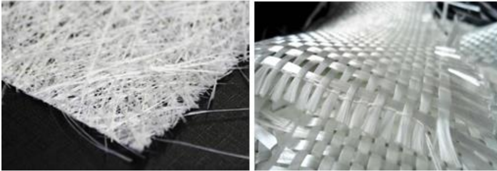
Figure 33: Chopped Strand Mat and Woven Roving
