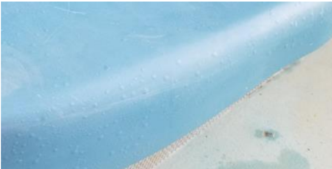
Figure 59: Gelcoat Blisters Needing Barrier Coat
