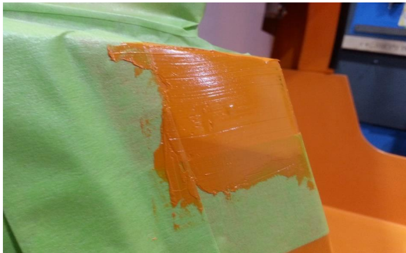
Figure 43: Applying Gelcoat Putty
