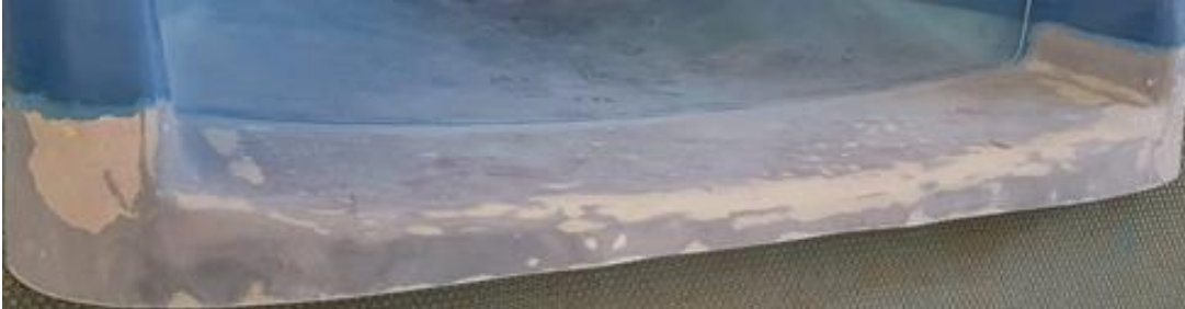
Figure 60: Sanded Gelcoat Ready for Barrier Coat
