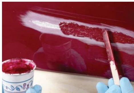
Figure 26: Vertical Surface Repairs
