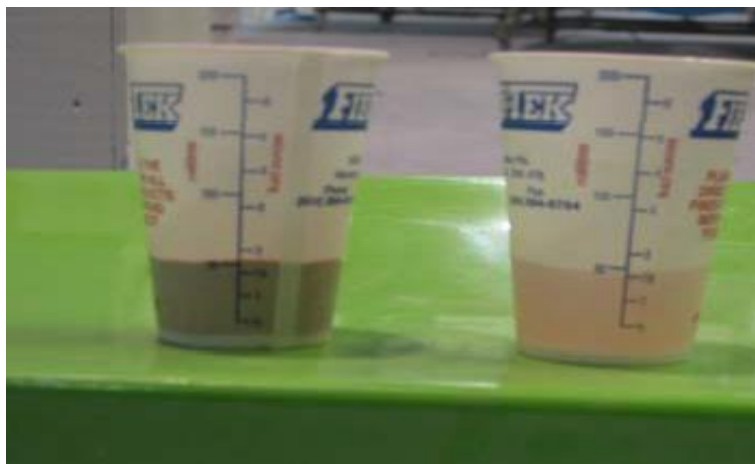
Figure 48: Pour Equal Gelcoat and Pro Patch Amounts
