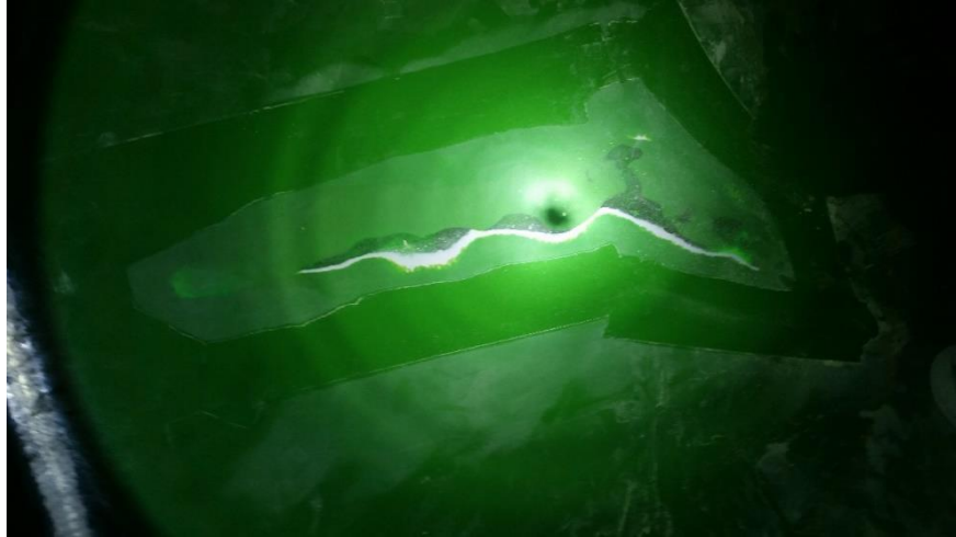
Figure 46: Sanded and Cleaned Putty on Fiberglass Repair, Inside
