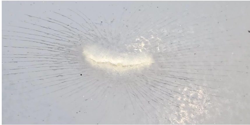
Figure 18: Dent in FRP
