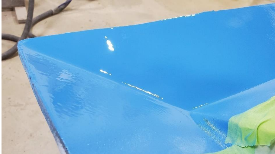
Figure 54: Spray the Entire Surface
