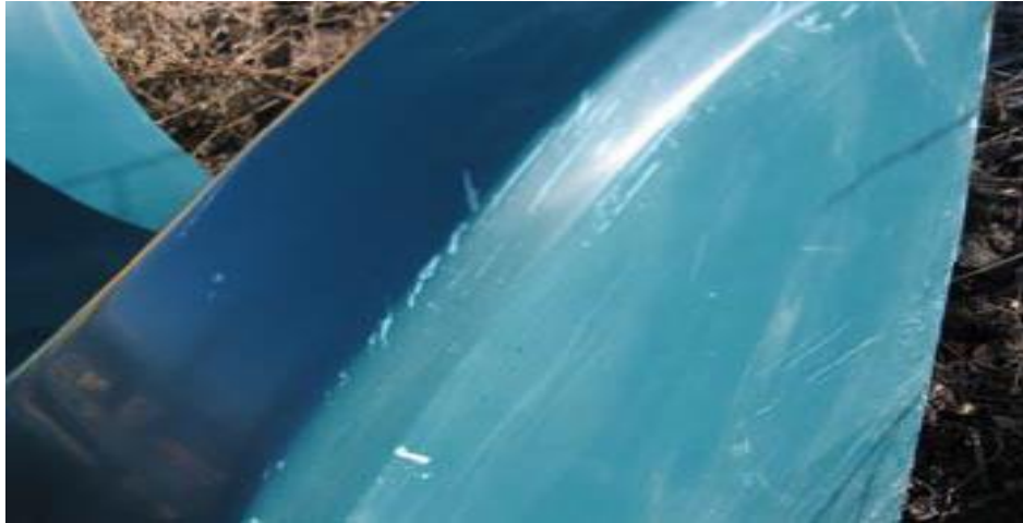
Figure 22: Scratches in Gelcoat
