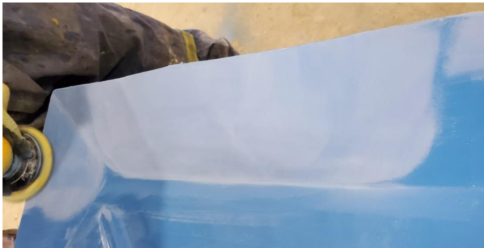
Figure 55: Sand with 400 to 600 grit Sandpaper
