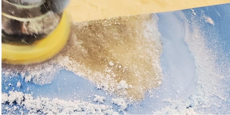
Figure 40: Sanding Fiberglass Repair
