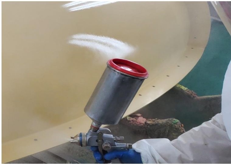
Figure 72: Spray in Controlled Area with Full PPE
