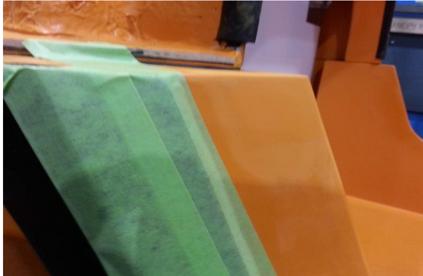
Figure 44: Sanded Gelcoat Putty Repair
