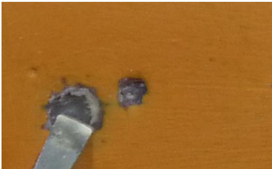
Figure 42: Defect for Gelcoat Putty Repair
